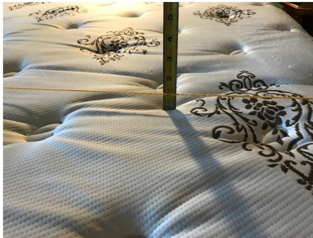
Showing the defect. If an impression, with a straight edge across the mattress, measure down showing the depth of the impression
